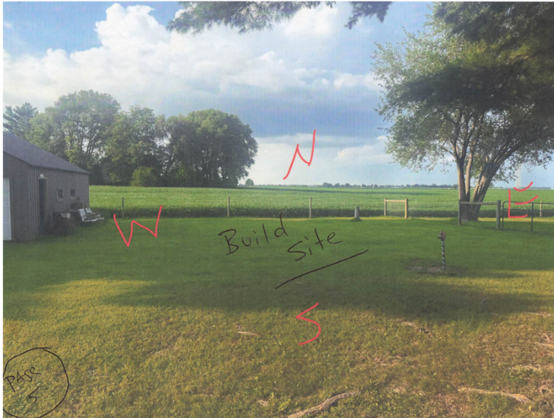
Figure 3. The proposed build site. Access to the structure must come from the south as the existing garage (west) and fence (east) would make maneuvering into and out of the structure impossible from any other direction. The spigot in the midground would make maneuvering more difficult if the proposed structure is made to comply with 15-ft minimum.
